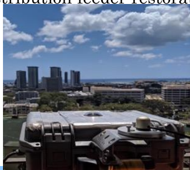
Recent pictures of HNEI's ground-based sky imager for minutes-ahead PV forecasting.
